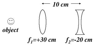
For the first lens  $1/s_{i1} = 1/f-1/s_{o1} = 1/30-1/30 = 0$ ,  $s_{i1} = infinity$ .  $s_{i1}$  becomes  $s_{o2}$  at -infinity. Thus,  $1/s_{i2} = -1/20+1/infinity = -1/20$ ,  $s_{i2} = -20$  cm. The image is virtual and 10 cm in front of the first lens. The magnification of for the system is  $M = (s_{i1}/s_{o1})(s_{i2}/s_{o2}) = (-infinity/30)(20/-infinity) = 2/3$ .
